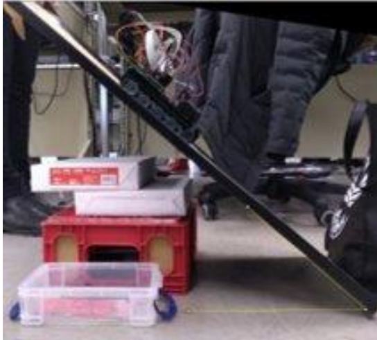
Figure 15: Ramp test with a maximum slope of 40 degrees.
