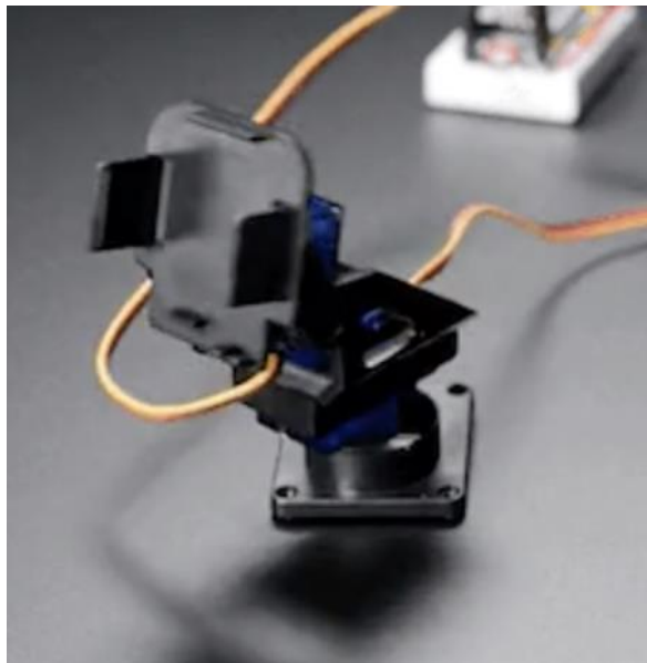
Figure 6: Camera mount structure with both the upper tilt and lower pan servos. (Adafruit, 2015)
